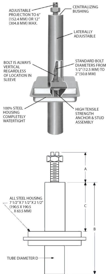
Anchor studs can be adjusted to protect above the floor from 0" to 12"(0mm to 304.8mm), depending on the bolt specified for the installation. The entire internal anchor assembly can be adjusted laterally as well as vertically to compensate for normal construction variances in both hole location and machine foot thickness.
