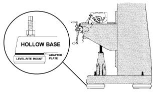
Designed for hollow bases as found on certain models of mills, lathes, grinders and other machines. Provides vibration control, leveling and support.
