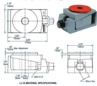
MOUNTING PLATE, TOP WEDGE, BOTTOM LIFTING WEDGE, AND BASE: 65-45-12 DUCTILE IRON. TENSILE STRENGTH: 65000 PSI (454.8 Mpa) MIN.
