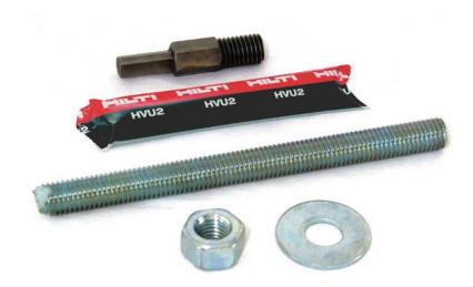
This system provides a superior method of heavy duty anchoring using a high strength adhesive to retain a threaded rod and other materials such as rebar in concrete or other masonry material. The system consists of an adhesive capsule containing the proper proportion of base resin, hardener and aggregate for the anchor, an appropriate length stud with washer and nut, and a drive unit to allow the stud to be inserted into a standard hammer drill.
