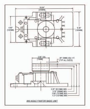
Pre-layout or core drilling is not required as the anchor holes are simply drilled through the mount base after installation. The use of the optional toggle clamp permits this to be accomplished even when overhanging machine components prevent access to the center or side anchor locations.
