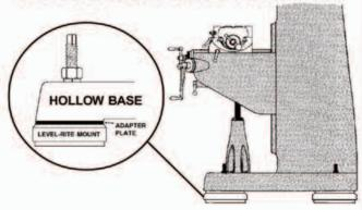
Designed for hollow bases as found on certain models of mills, lathes, grinders and other machines. Provides vibration control, leveling and support.
