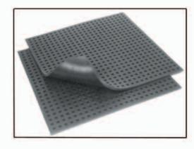
The smooth edge design of the low cost oil-resistant UNISORB NEOPRENE PAD prevents oil, grease, and dirt from accumulating beneath the load-bearing surface of the pad. Available in 18" X 18" X 5/16" (457.2mm X 457.2mm X 7.9mm). Stiffness is 60 durometer.
