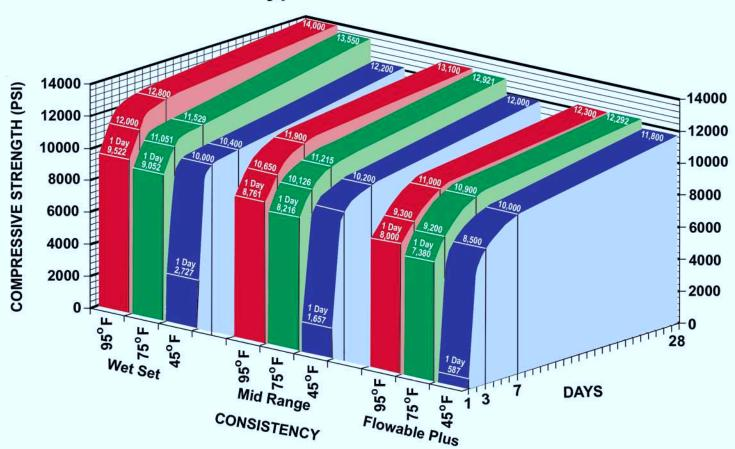
Unisorb WTF Non-Shrink Grout is a cement based precision grouting product, specifically formulated to develop ultra high strengths. Blended cements, graded sands, and a performance enhancing super plasticizer make a grout product that will be flowable with the addition of a minimum amount of water. The result is a cementitious grout that is surprisingly user friendly and will rapidly develop very high compressive strengths.
