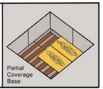
A mud mat is poured, then rows of base isolation material are placed, with the air gap integrity protected by sheets of treated plywood. This allows more weight to be concentrated on the base material, thus driving the pad loading up and the natural frequency down.
