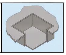
This method of construction is used where soil conditions are less than ideal, or when it is desirable to provide a positive seal against contaminates reaching the sub soil. This creates a "socket" for the isolation material and inertia block foundation to be placed.
