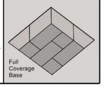
IB-500 foundation isolation pad materials are suitable for direct exposure to wet concrete, however the joints must be sealed with Unisorb IB-500 Seam Tape to prevent the incursion of fluid concrete during pour. It is also advisable to place a Unisorb Poly Pit Liner inside the lined pit to assure that no "short circuits" occur.
