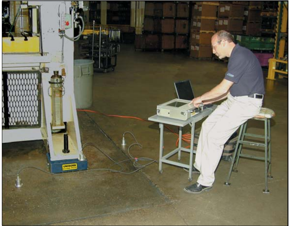
PERFORMING MULTI-CHANNEL VIBRATION SURVEY
